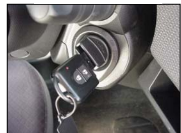
Emergency mechanical key in use
